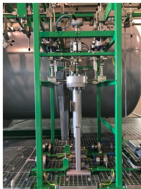
This type of filter can be designed for different types: the removal of solid particles and the removal of liquid particles (coalescing filters). The filtering elements can be used in all types of metallic or plastic materials, polyester, felt, glass microfiber.
