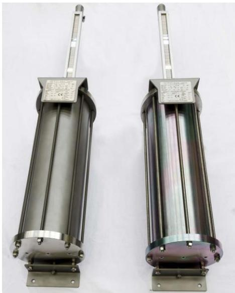
The lower part of the cylinder is used to contain the sample for Analyzer validation, while the upper one is used for moving the piston and the consequent sample pushing to the Analyzer.
